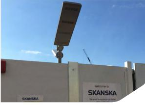
The ProTemp is a powerful and versatile solar-powered light mounted on a 1189kg steel-encased concrete base with a 5.4m telescopic mast. As a standalone unit it can be easily transported to site and moved into position with a forklift.
